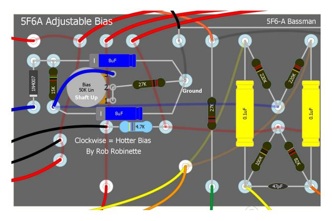
The bias pot wired as a variable resistor and 27k resistor replace the 56k resistor above.
